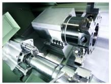
The DANOBAT TCN 4 axes horizontal lathe has been designed to create new high standards in turning of railway axles with precision and high productivity, with the possibility of roughing operations for forged train axles.
